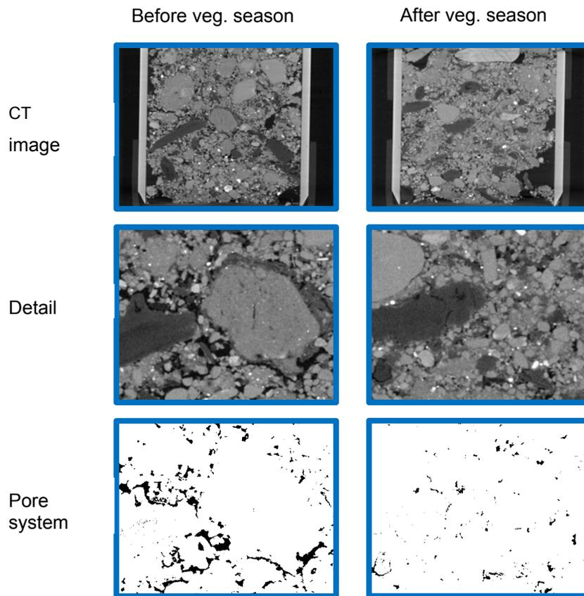
**Figure 3.** Vertical sections of the three-dimensional X-ray tomographs of two different samples taken from the filter layer of the bioretention cell before and after vegetation season. Original, detailed and segmented 2D sections are displayed in upper, middle and bottom row. In this case the macroporosity decreased from 7 to 2 %.
