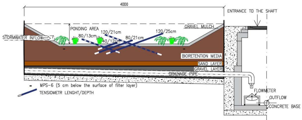
**Figure 1.** A schema (longitudinal section) of the bioretention cell.
