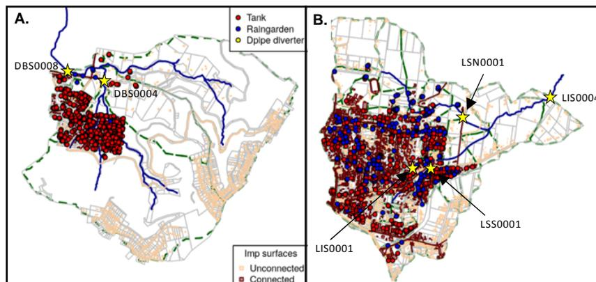
Figure 1. Intervention catchments showing impervious areas and the nested distribution and type of installed SCMs. A. Dobsons Creek catchment including DBS0008 and DBS0004; B. Little Stringybark Creek catchment including LSN0001, LIS0001, LSS0001 and LIS0004.
