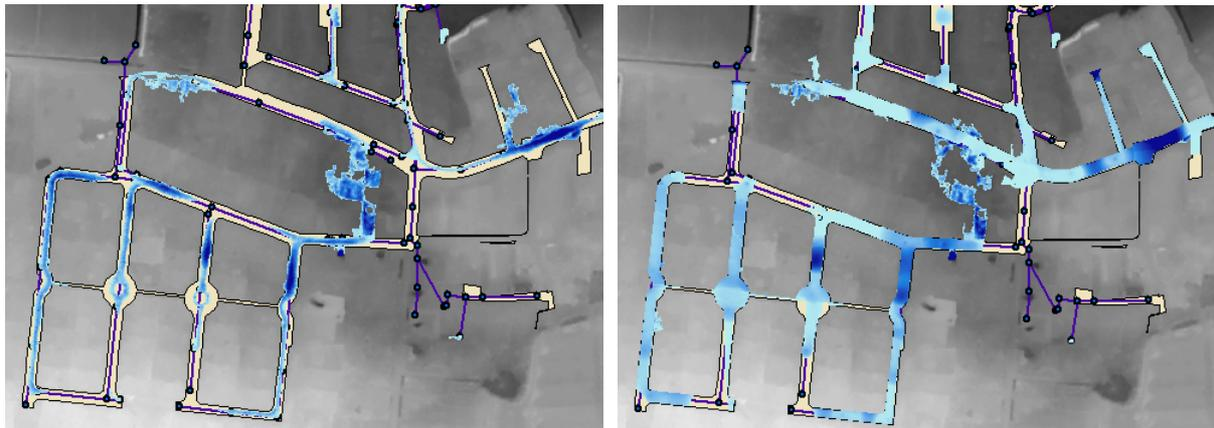
Figure 3: Flooding area without (left) and with (right) impressed streets
