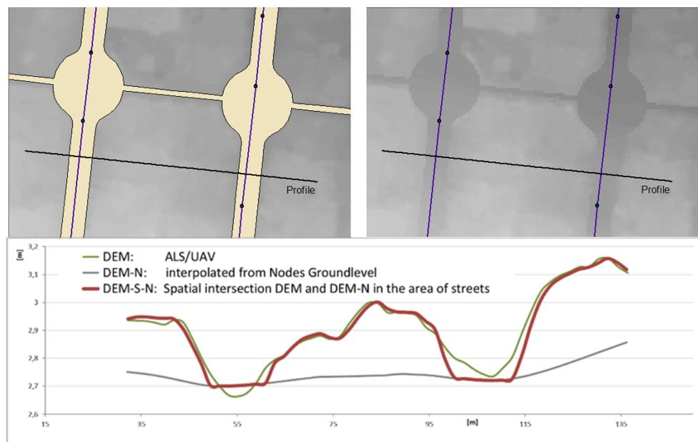
Figure 2: Intersection of DEMs for impressing streets with individual groundlevels of nodes
