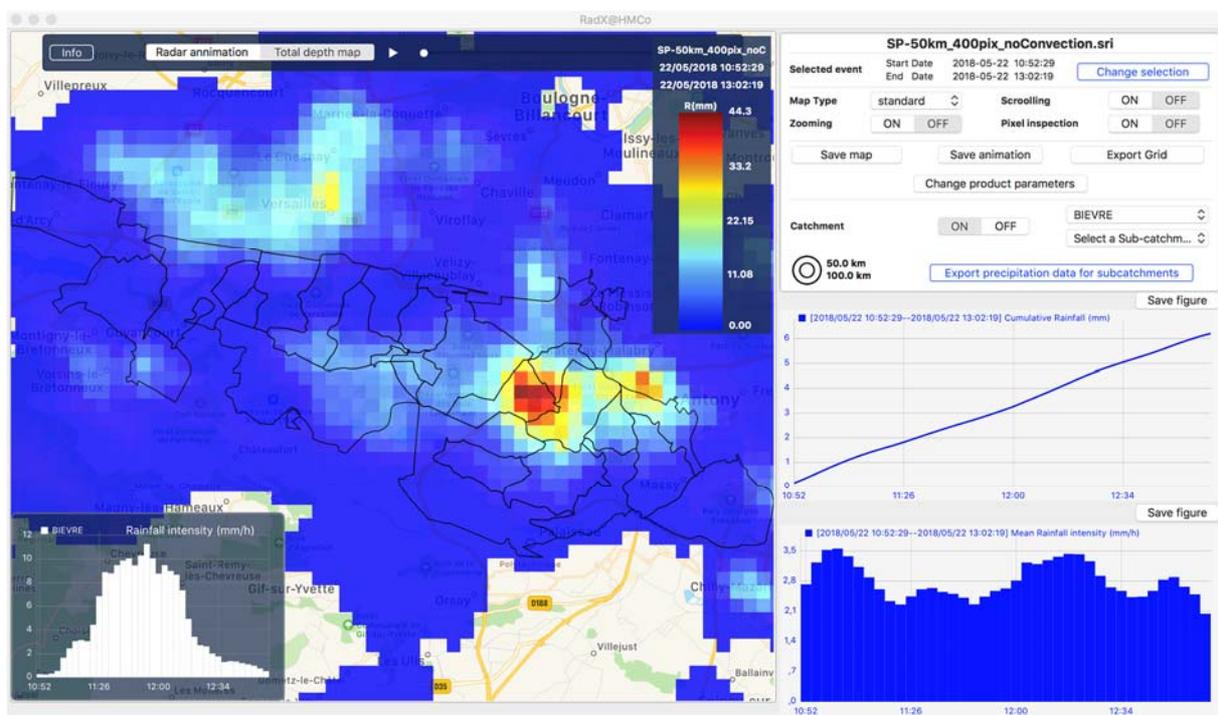
Demonstrator of the ENPC X-band Radar Platform, with the zoomed view over the Bièvre Valley on May 22, 2018, 11AM-1PM UTC. The hot spot corresponds to 26 mm of 2h cumulative rainfall over the BIEV sub-catchment, situated just in between the three rain gauges (JOUY3, SYGAM and VER1 sub-catchments), the maximum per pixel is above 44 mm. This is a very heterogeneous event, only 6 mm were obtained over the full rainy area of the X-band radar observations (up to 100 km radius around the ENPC).
