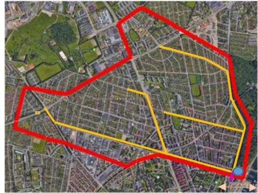
Fig. 1: Trøjborg Catchment with detention tank at the blue circle, yellow main pipes and purple connection to neighbouring catchment
