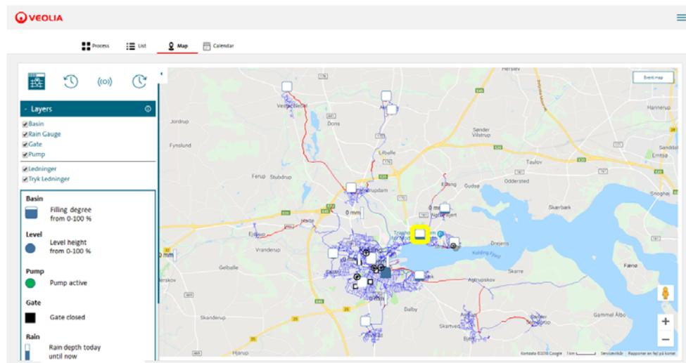
Figure 3: Basic live view of the sewer network (SewerView). In yellow marking the control algorithm indicates a possible overflow within the forecast horizon at a basin in the northern part of the sewer network.
