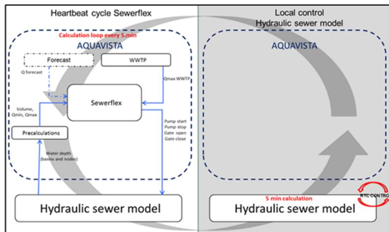
Figure 2: The Sewerflex MPC test environment. Every 5 min the hydraulic sewer model (to the right) is paused in order to extract water depths from the model. These are used to calculate inputs for the Sewerflex MPC. When setpoints have been calculated by Sewerflex (to the left) they are sent back into the hydraulic sewer model and the calculation continues for another 5 min.
