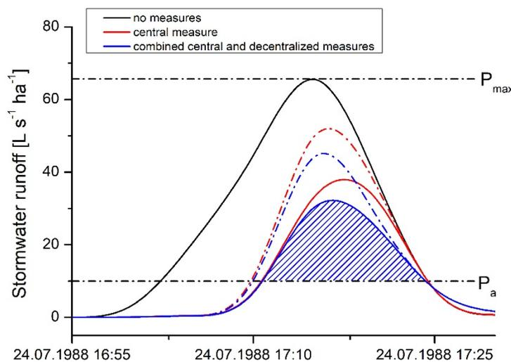
Figure 2: Stormwater runoff  $P(t)$  to urban river for three scenarios (case study 1). The hatched area exemplifies the integral in equation (2) for one scenario. The dashed lines show the effect of a reduced retention volume of the central measure by 25 %.
