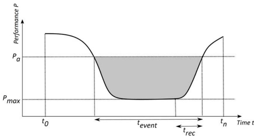
Figure 1: Schematics of equ. 2, adapted from Mugume et al. (2015). The grey area shows the integral in equ. 2.
