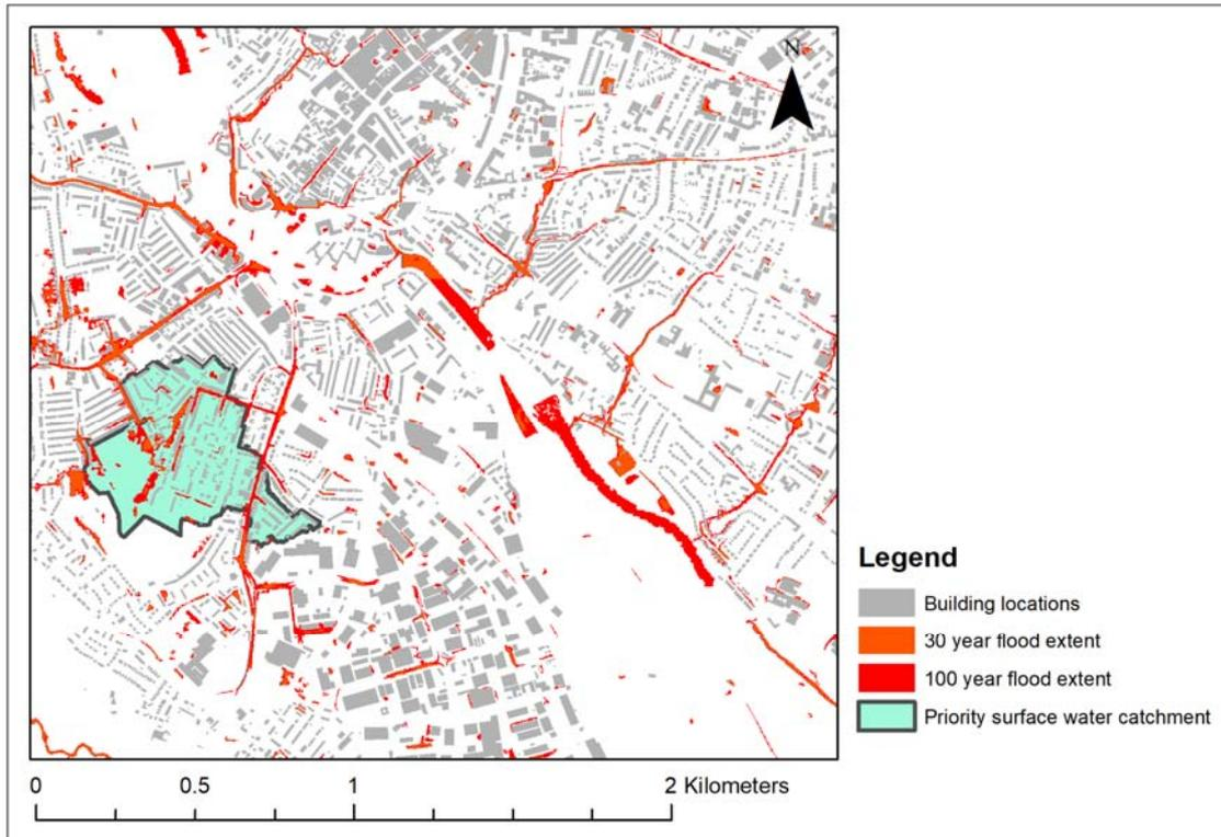
Figure 1: Snapshot of prioritising a surface water catchment based on flood risk using the GIS screening tool
