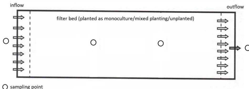
Figure 1: Experimental design of a single filter bed
