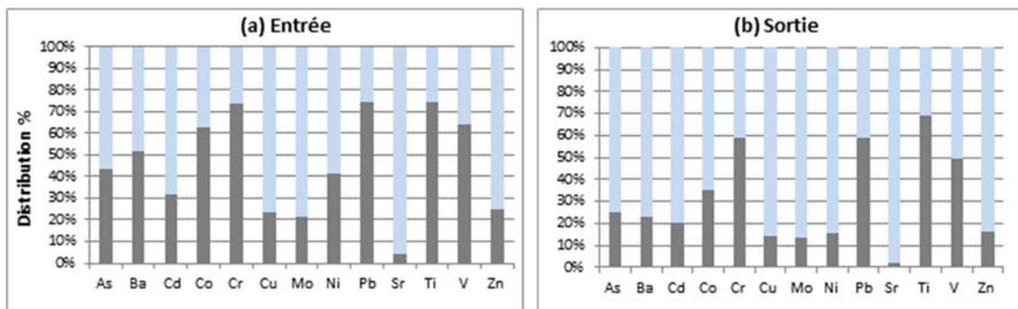
Figure 2. Distribution of metals between the dissolved and particulate phases of the dry basin: (a) inlet (b) outlet
