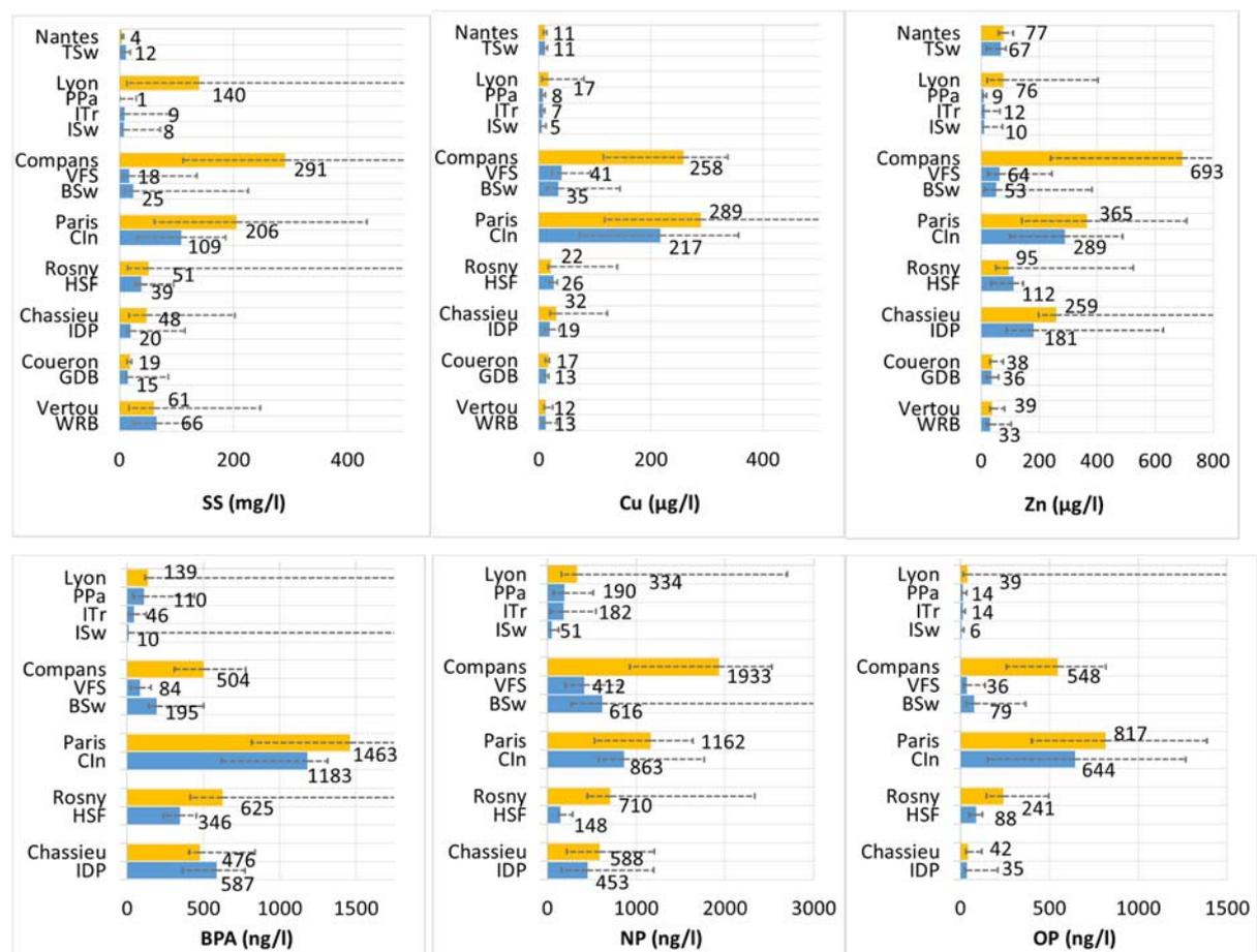
Figure 1 : D10, D50 and D90 of event mean concentrations (EMCs) measured in the runoff from the different study sites (inlet in yellow and outlet in blue)
