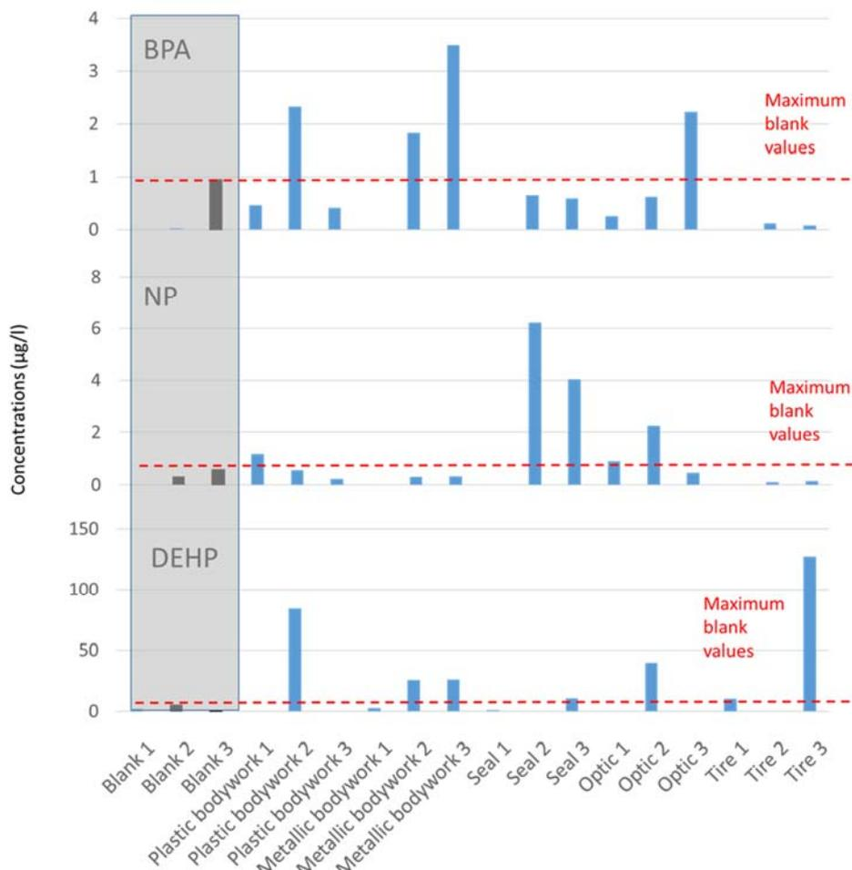
Figure 2 : Concentrations of BPA, NP and DEHP ( $\mu\text{g/l}$ ) in synthetic water after leaching of vehicle components
