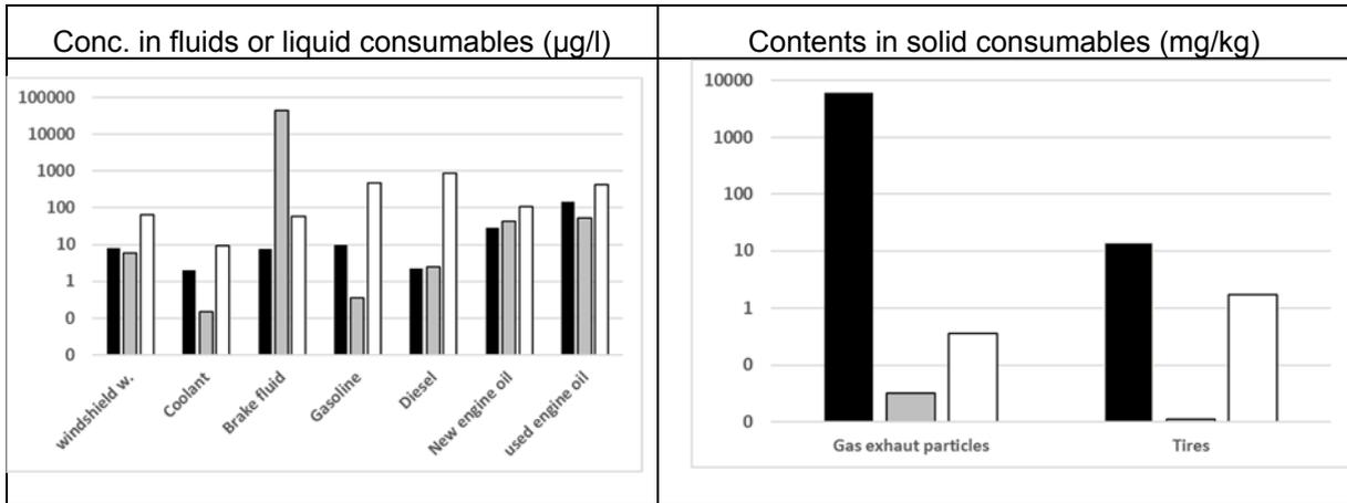
Figure 1 : Mean concentrations or contents of PAE ( $\Sigma 6$ , black), BPA (grey) and APnEO ( $\Sigma 7$ , white) in different automotive fluids or consumables
