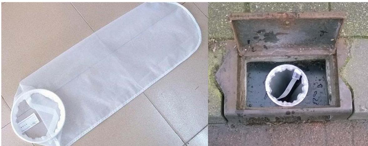
**Figure 1.** a Filter bag with a diameter of 18 cm and a length of 50 cm. b Experimental setup.
