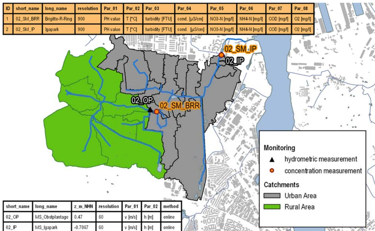
Figure 1 : Location of the measuring points including representation of the measured parameters
