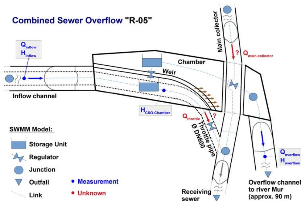
**Figure 1:** The structure of the CSO R-05, the observed properties at their installed measurement locations and the used SWMM model discretization
