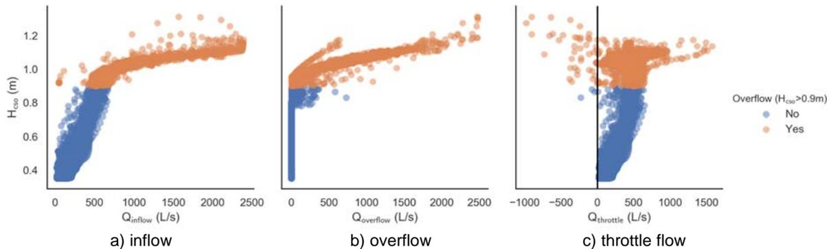
**Figure 2:** Comparison of the flows of the CSO R-05 against the water level of the CSO chamber for a period of 30 months (2009-2011). The data was subdivided into data points occurring during overflow events (orange) and periods without overflow (blue) for better visualization. The weir crest height in the overflow chamber determines the occurrence of an overflow and corresponds to a water level  $H_{cso}$  of 0.9 m.
