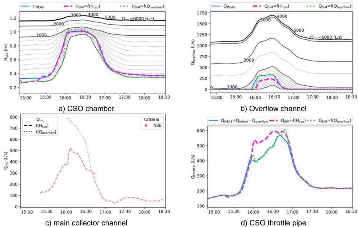
**Figure 4:** Comparison of the measured data (blue) with the simulation results based on constant main collector flows (steps of 1000 L/s (thick black lines) and of 500 and 100 L/s (thin black lines) and on the estimated main collector flow (magenta: optimized for  $H_{CSO}$ , green: optimized for  $Q_{overflow}$ )
