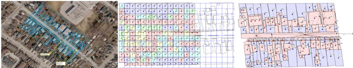
Figure 3 A 1.64 ha site and the two modeling approaches (grids and homogeneous subcatchments).
