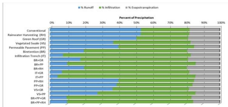
Figure 3 Water balance of different combinations of LID alternatives.
