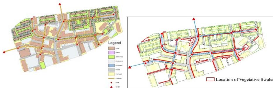
Figure 2 Sub-catchments modified with LIDs and locations of swales.
