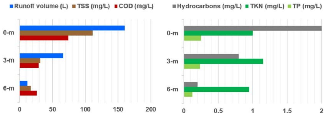
**Figure 2.** Comparison of the median runoff volumes and pollutant concentrations in runoff collected 0 m, 3 m and 6 m from the highway edge on the vegetated slope.
