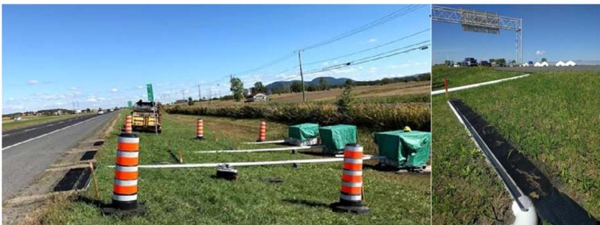
**Figure 1.** Pilot highway runoff collection system with gutters and collection tanks, and view of 3-meter gutter.
