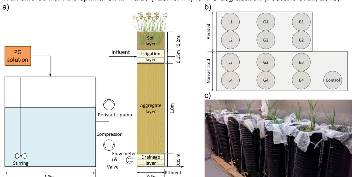
Figure 1. A a) cross-sectional and a b) top view illustration of the setup utilised as well as c) the finalised columns.
