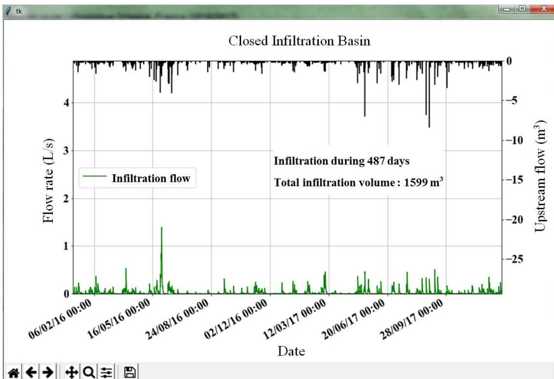
Figure 2. Simulated infiltration flowrate in the closed infiltration basin during 2 years
