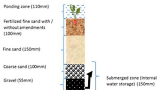
Figure 1. Set-up of biofilter columns
