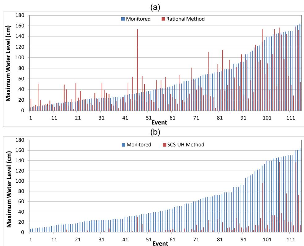
Figure 2: Comparison between maximum water levels monitored and calculated with (a) Rational Method (b) SCS-UH Method (OSD-C)
