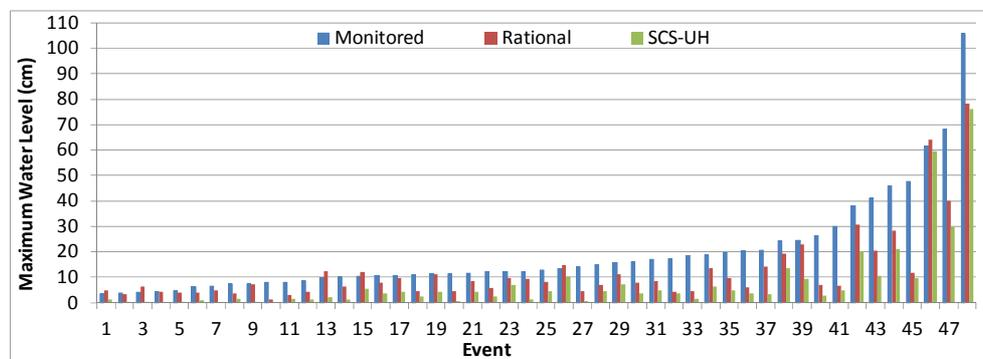
Figure 1: Comparison between maximum water levels monitored and calculated with theoretical methods (OSD-H)
