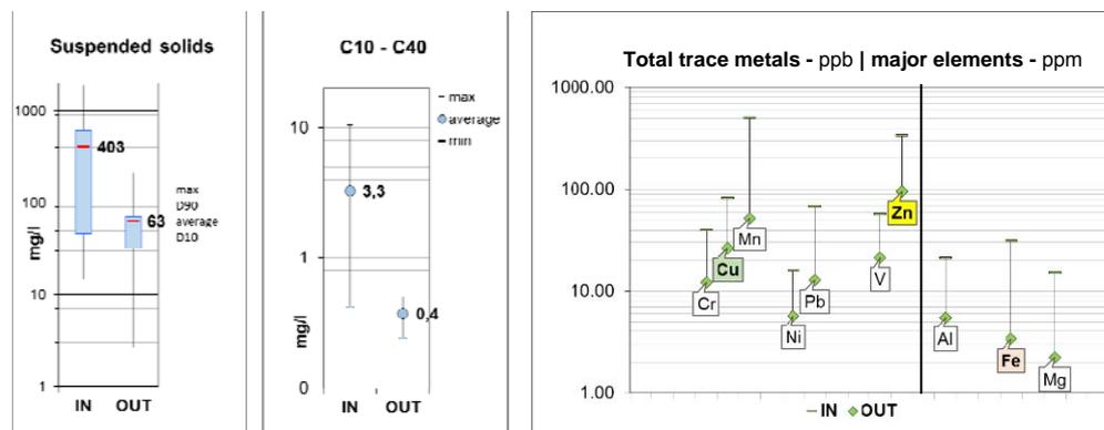
**Figure 3:** Water quality data of influent (runoff) and effluent. Suspended solids (A) data are based on 14 events. Total hydrocarbons (B) and average of total metals (C) are based on 4 events.
