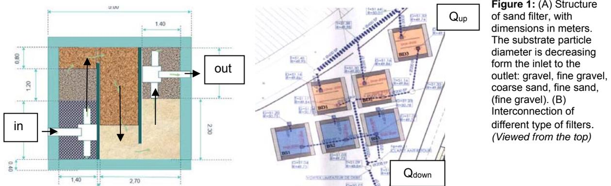
**Figure 1:** (A) Structure of sand filter, with dimensions in meters. The substrate particle diameter is decreasing from the inlet to the outlet: gravel, fine gravel, coarse sand, fine sand, (fine gravel). (B) Interconnection of different type of filters. (Viewed from the top)
