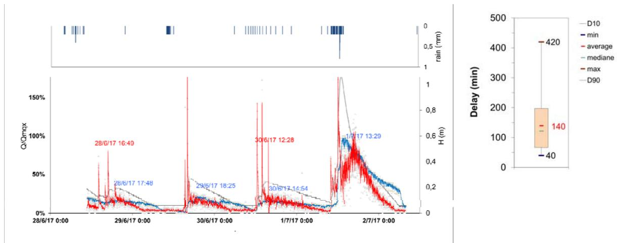
**Figure 2:** (A, left) Example of inflow (red) and outflow (blue) of the first series of filters and (B, right) the delay of peak flow for the period June – September 2017 estimated for 14 events. Smooth grey line indicates the water level at the entrance of the first filter.
