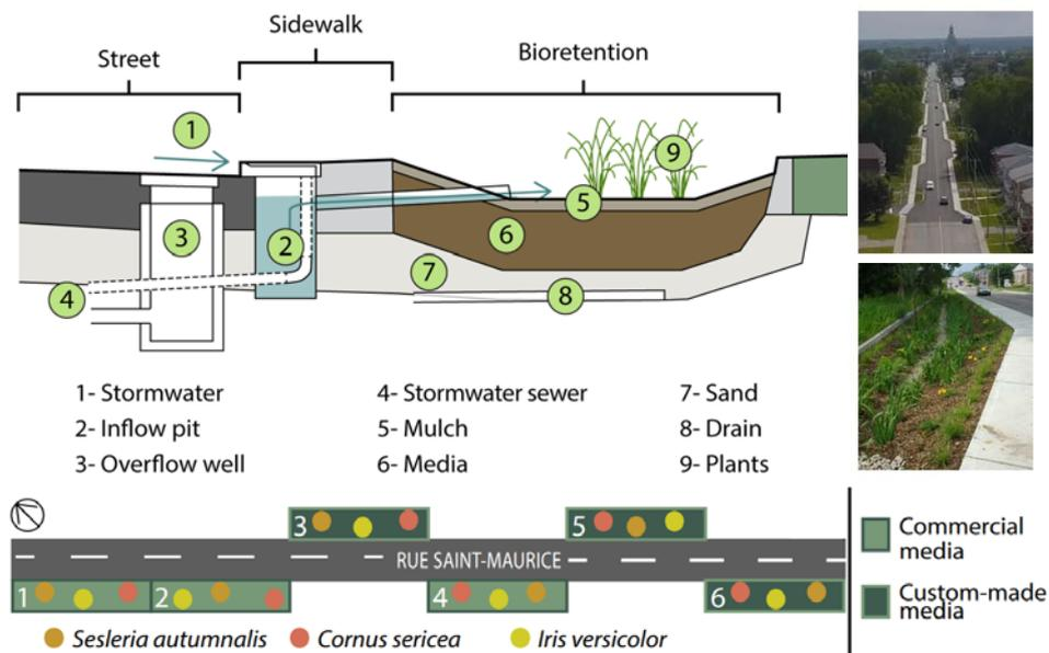
**Figure 1.** Top. From left to right: sectional drawing of a BRC; Saint-Maurice Street after BRC implementation; view of BRC with *Sesleria autumnalis*, *Hemerocallis* 'Stella de Oro' and *Iris versicolor*. Bottom: distribution of 6 BRCs on the street with location of root cameras and monitored plant individuals.
