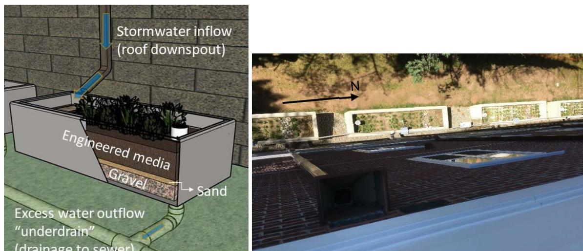
Fig. 1. Typical above-ground bioretention planter configuration (left); test site at Stevens Institute of Technology (right).
