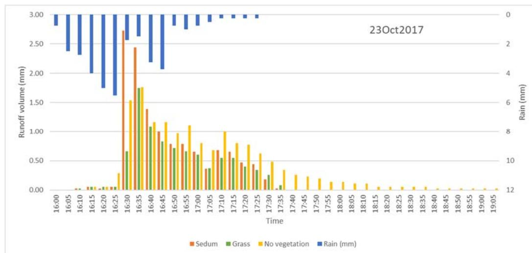
Figure 2 – Runoff and rain volume of the green roof
