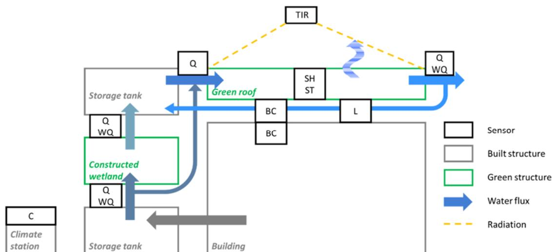
Figure 1: Schematic representation of green roof setup and measurement configuration. Sensor groups are C – climate, Q – flow, WQ – water quality, L - lysimeter, SH – substrate humidity, ST – substrate temperature and TIR – Infrared surface temperature
