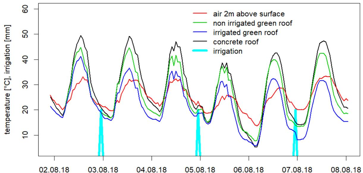
Figure 2: Simulated surface temperatures of non irrigated and irrigated green roof, concrete roof and reference air temperature 2 m above ground for the period 02. – 08.08, with climate forcing data from Dresden Klotzsche meteorological station.
