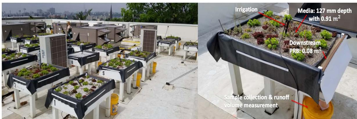
Figure 1 North Building green roof experiments (left) and tray assembly (right)
