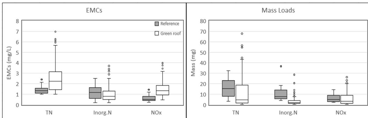
Figure 2 EMCs (left) and mass loads (right) of total nitrogen, inorganic nitrogen and NO<sub>x</sub> from pilot scale ungreened reference roofs and green roofs.
