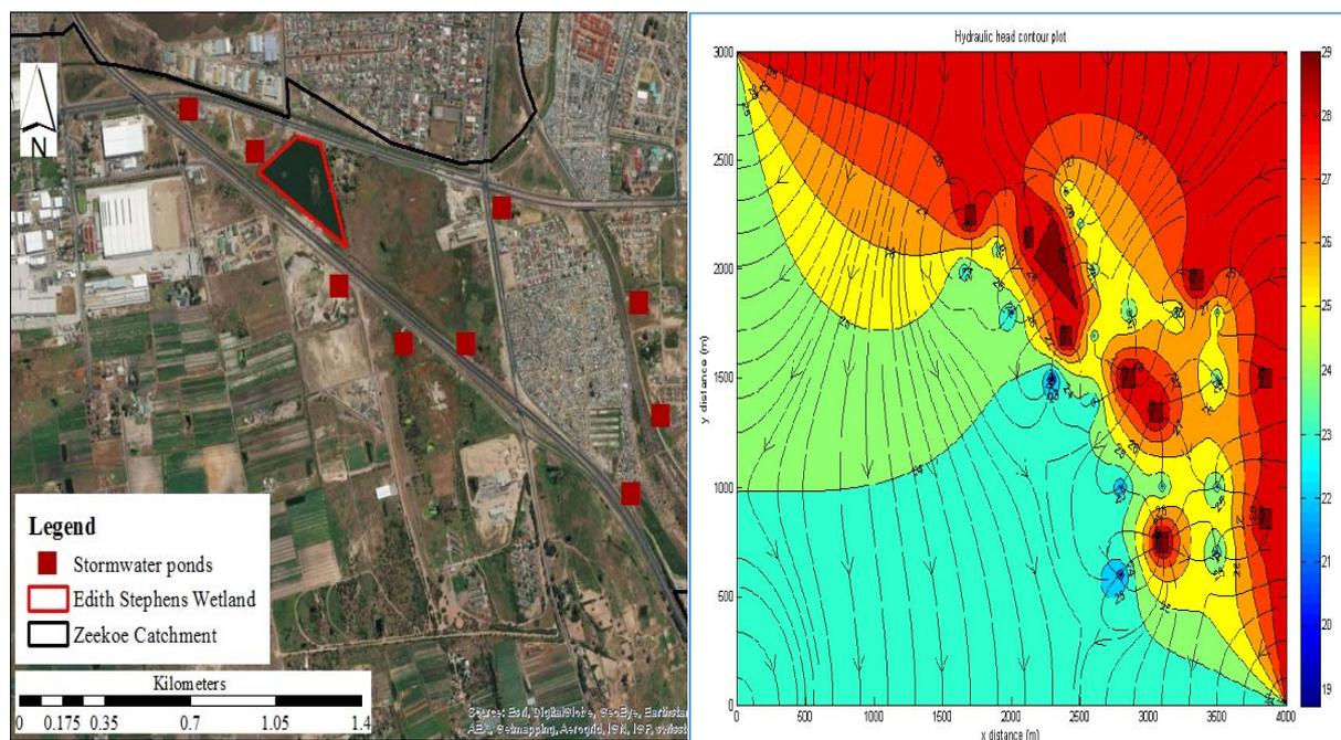
**Figure 3 Modelled phreatic flow fields from the stormwater ponds to the boreholes**
