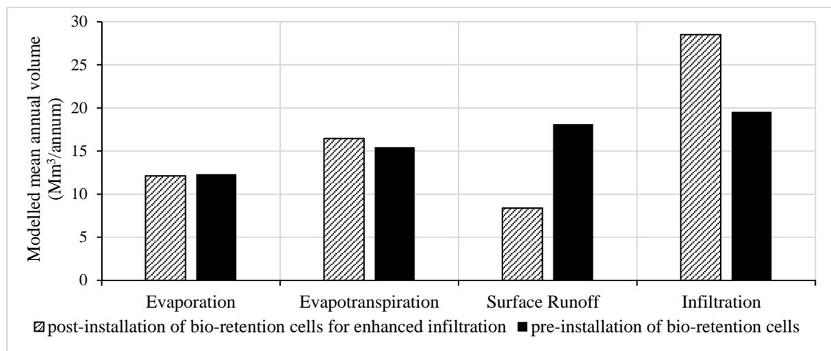
**Figure 2 Comparison of existing and post-modification to bio-retention**
