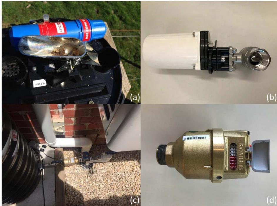
Figure 2. (a) Rain gauge, (b) solenoid valve for pre-storm discharge and baseflow release, (c) and (d) shows water meter to monitor end-use and active discharge through valve.
