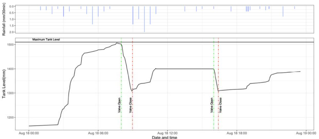
Figure 3. 24-hour trace plot for rainfall (top) and rain tank volume (bottom). Vertical dot lines indicate valve opening and closing for pre-peak discharge.
