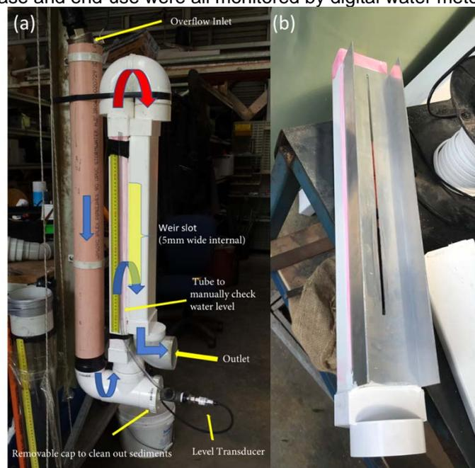
Figure 1. Schematic representation of inflow and overflow weir box (a) and internal rectangular weir (b). Blue and red arrow in (a) represent flow through weir and overflow respectively.
