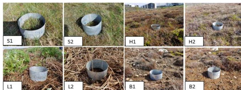
Figure 1 Infiltration rings in four vegetation covers: Grass swale (S1, S2); Heath (H1, H2); Lupine (L1, L2); Barren (B1, B2).
