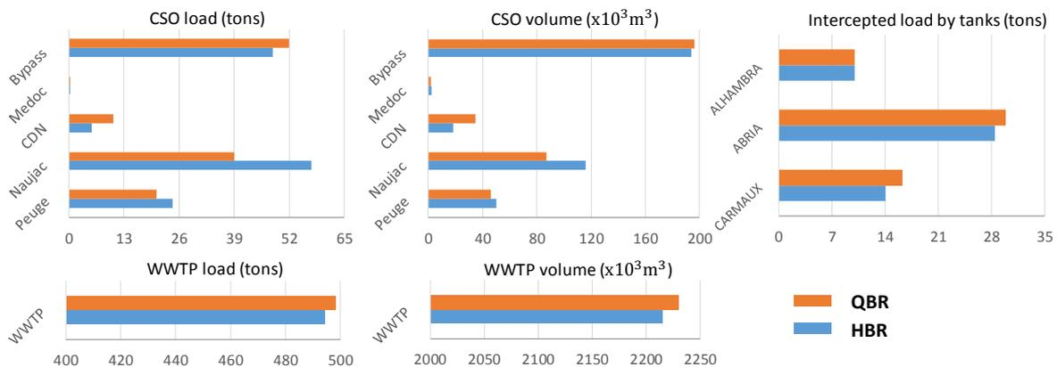
Figure 4. Total TSS loads and water volumes at different outlets together with intercepted loads by all the tanks from four CSO events.
