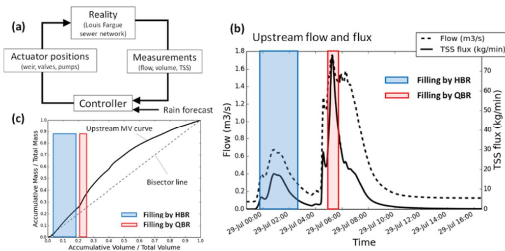
Figure 2. a) Summary of RTC workflow; b) Illustration of filling periods by two strategies over flow and TSS flux plots (upstream of the tank); c) Same illustration over the MV curve plot (upstream of the tank).
