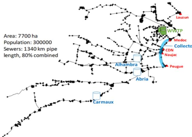
Figure 1. The sewer network with important locations for control.
