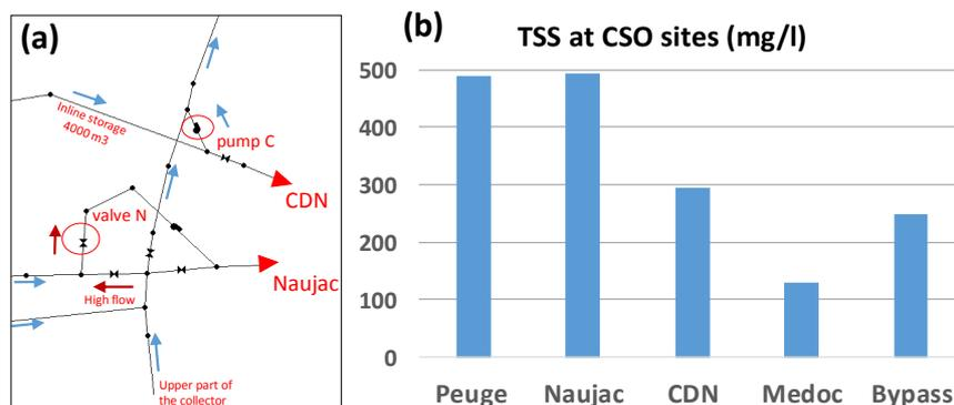
Figure 3. a: Actuators at the interceptor controlled by QBR; b: Mean TSS values from four CSO events with HBR.
