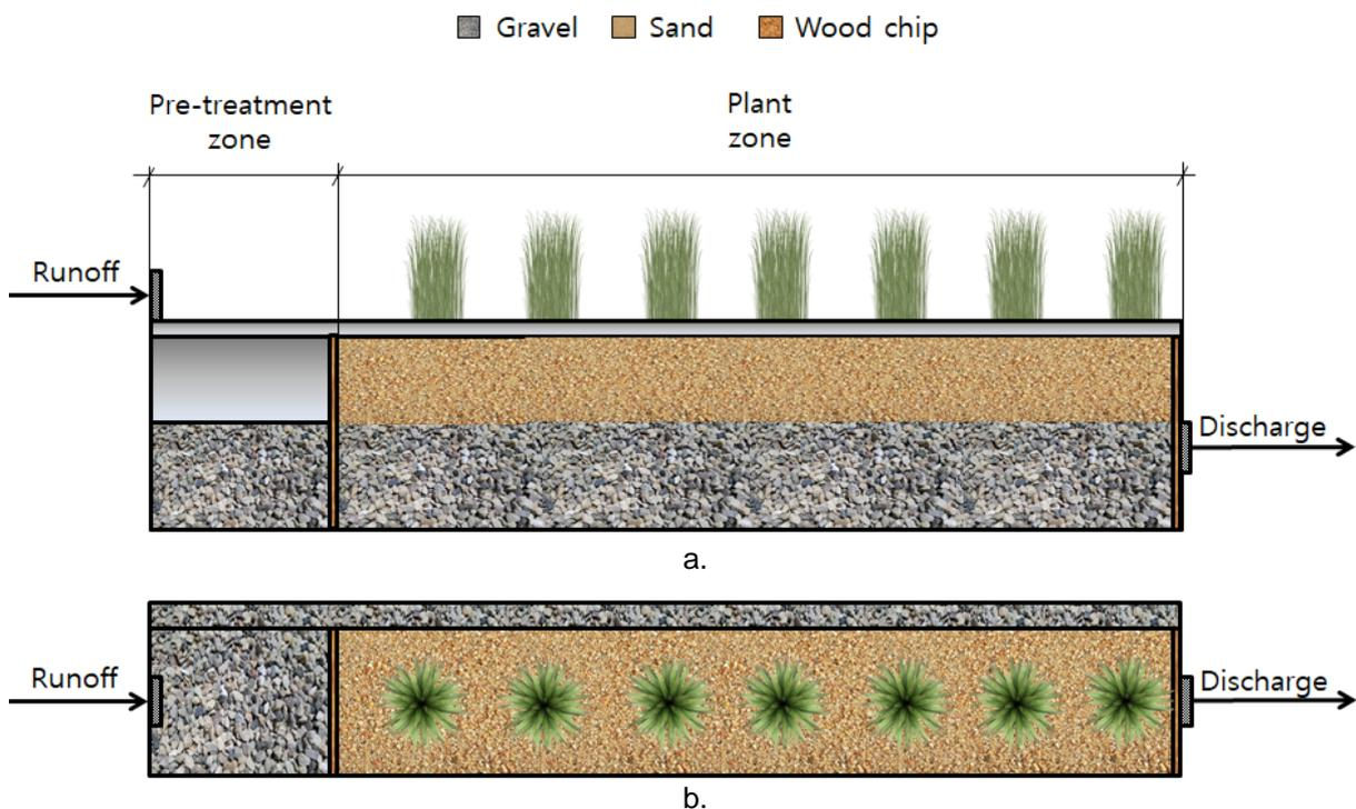
Figure 1. Schematic diagram of SHSSF CW: a) Side view b) Top view
