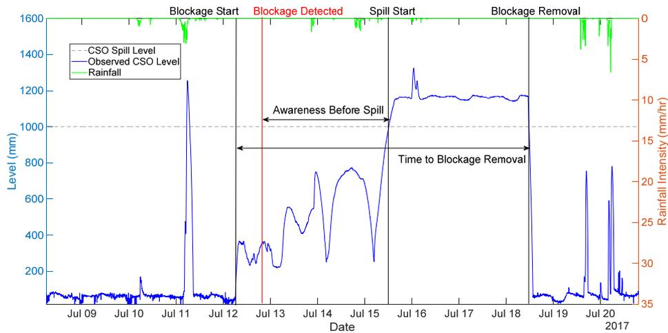
Figure 1 Results obtained by the detection system during a blockage event
