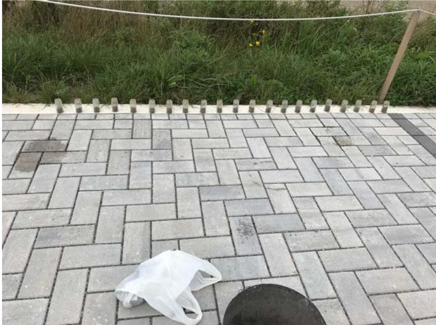
Figure 1: Weighted sediment in jar ready to be applied over the joint.
