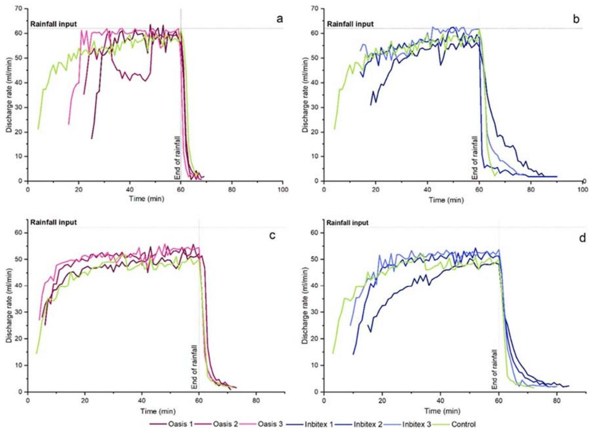
Figure 2. Discharge rate curve. (a, c) OASIS 1st and 9th event. (b, d) Inbitex 1st and 9th event
