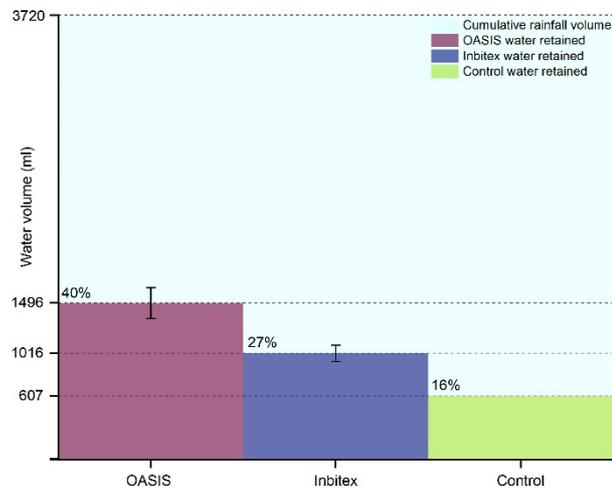
Figure 3. Water retention performance of OASIS, Inbitex and Control rigs
