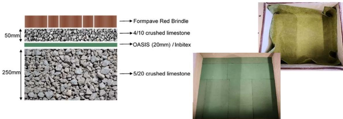
Figure 1. Schematic layout of PPS designs (left), installation of water barrier/treatment systems (Inbitex (top right), OASIS (bottom right))
