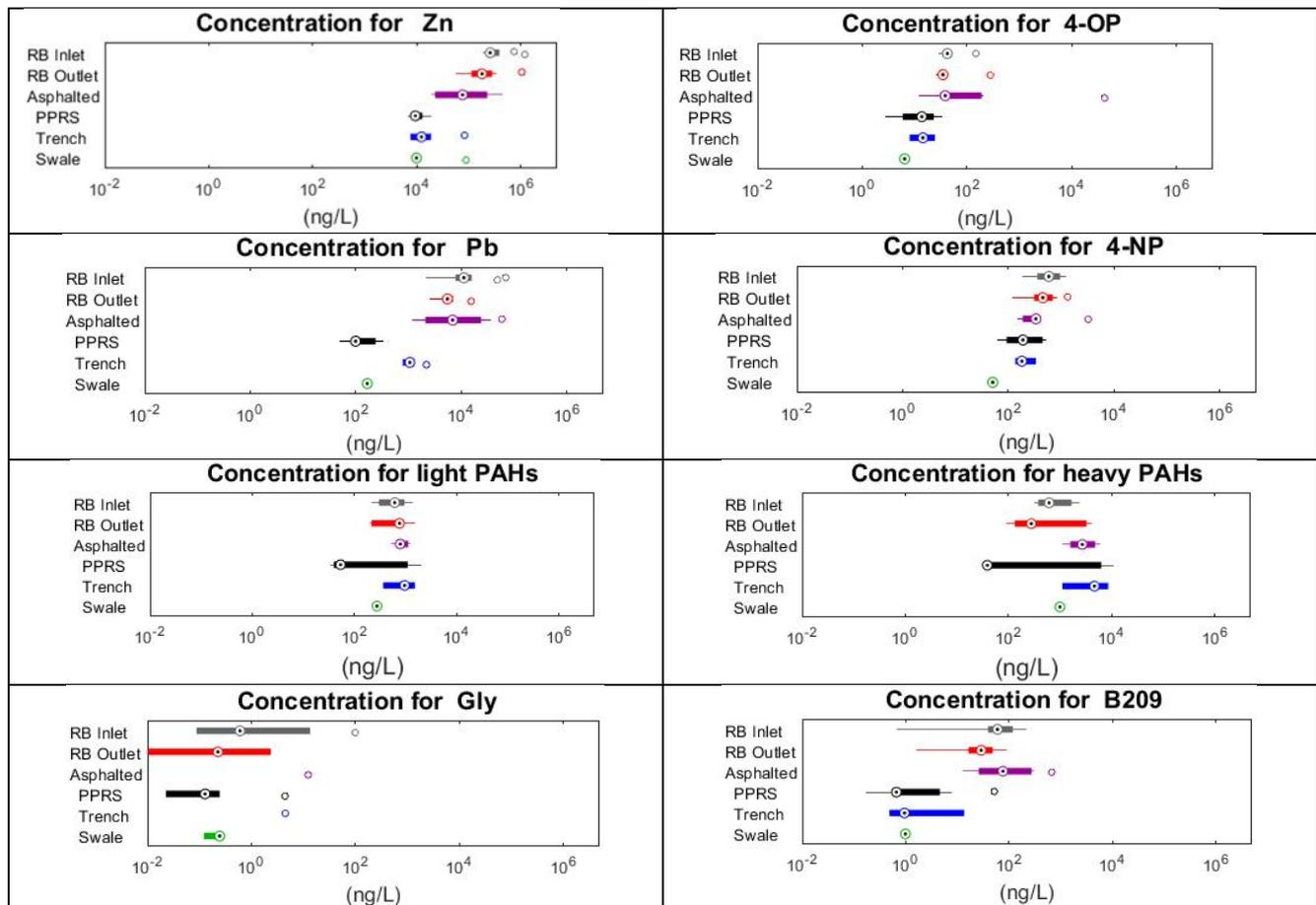
Figure 1 : boxplots of concentrations for micropollutants at the outlet of the source control systems compared to the reference (asphalted parking), and at the inlet/outlet of the retention basin
