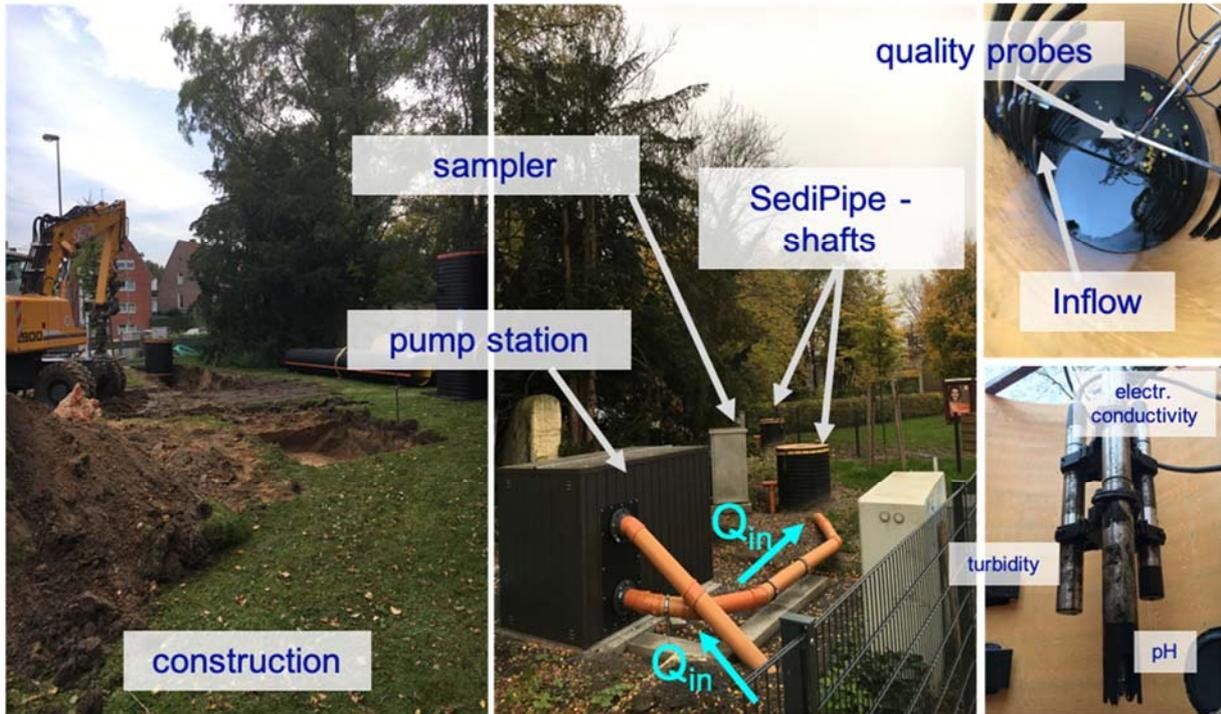
Figure 1: Monitoring station "Am Stadtgraben" (left: construction site, center: pump station, SediPipe-shafts and sampler; top right: Arrangement of the quality probes in the starting shaft; bottom right: Quality measuring unit after first event)
