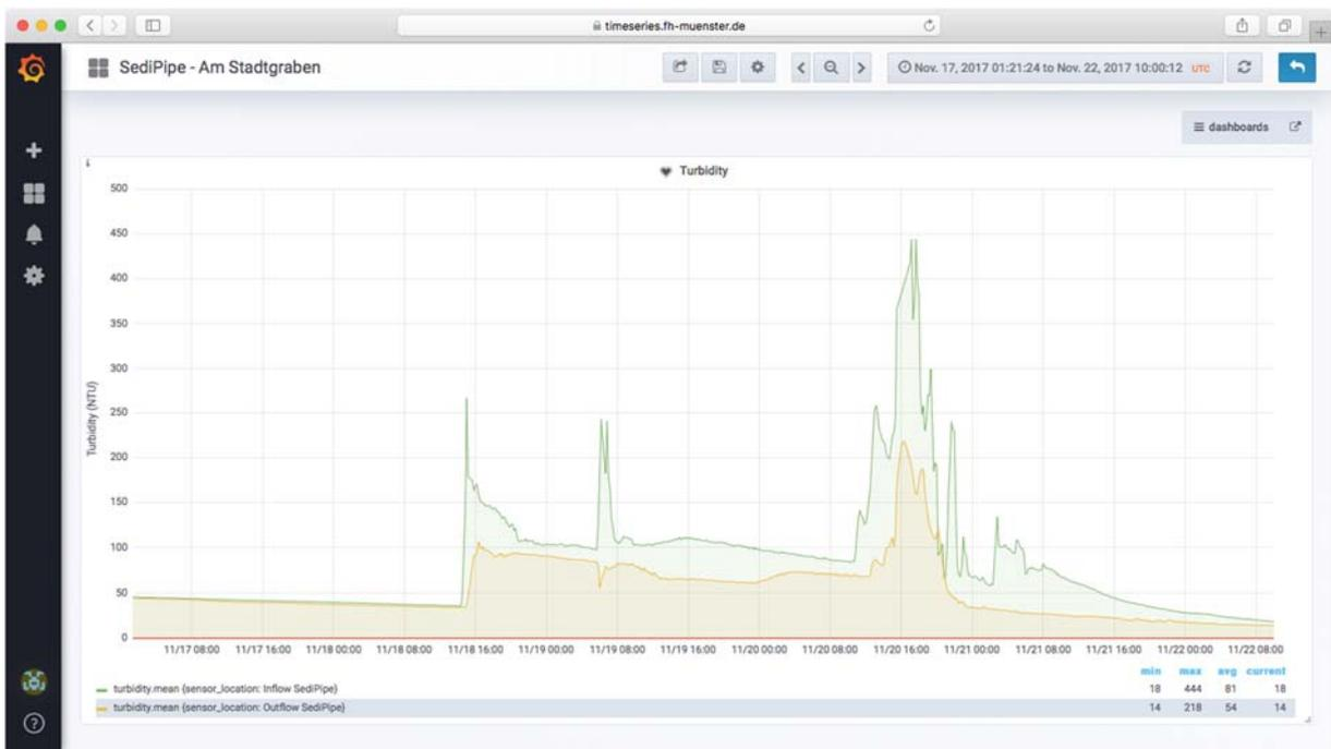
Figure 2: Web-based visualization of measurement data of site "Am Stadtgraben" (green: turbidity signal at the inflow; orange: turbidity signal at the outflow)
