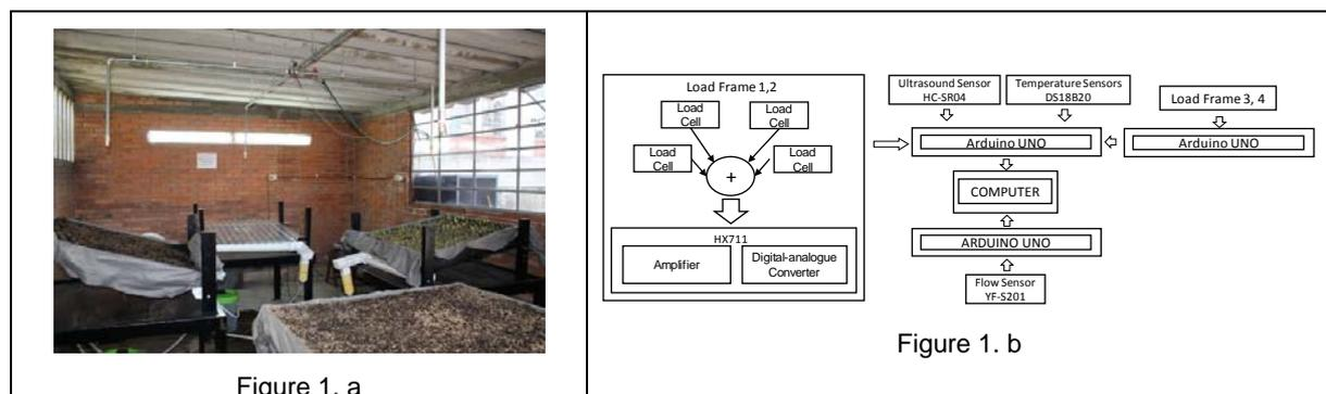
Figure 1. Experimental assembly and block diagram of the data acquisition system.
