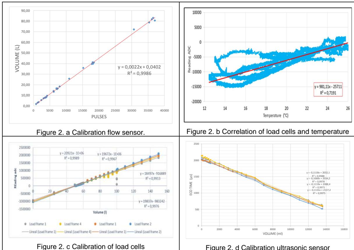
Figure 2. Calibration curves for the sensors of the experimental assembly.
