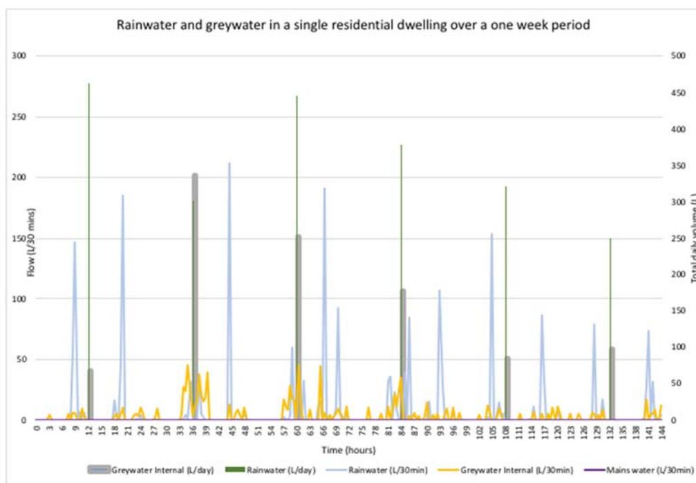
Figure 1. Example of smart metering output from a Fremantle residence maximising alternative water sources
