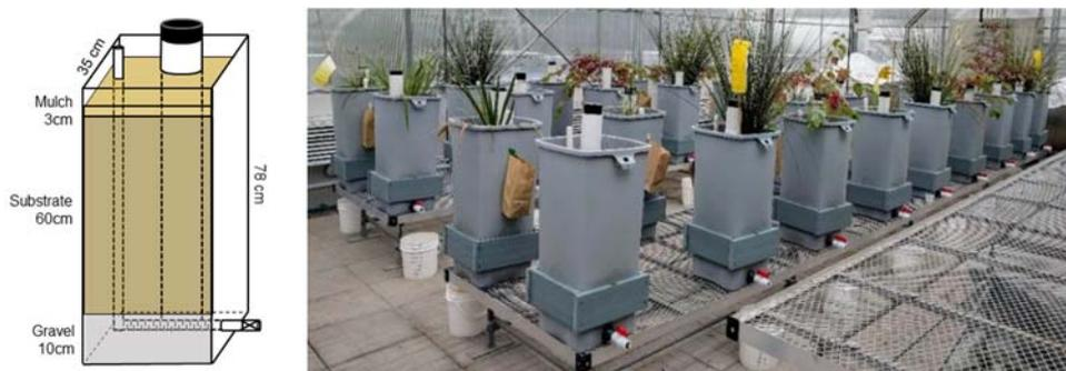
Figure 1. Design and layout of mesocosm-size bioretention cell experiment.
