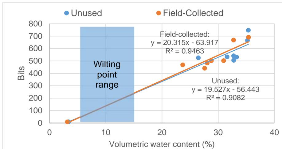
Figure 2. Calibration curves from Calibration 2 for unused and field-collected filter media volumetric water content.
