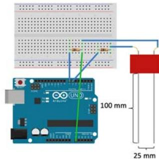
Figure 1. Basic circuit diagram of Arduino-based sensor node with soil moisture sensor (red block with grey electrodes). Power source, SD card reader, and 3G module not shown.
