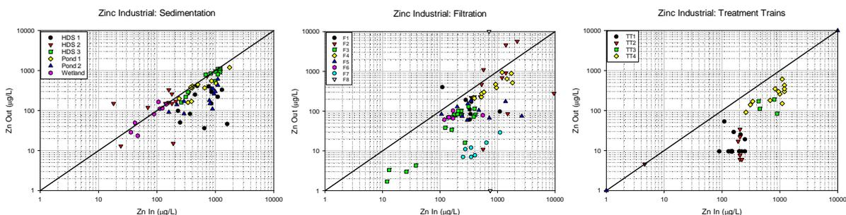
Figure 2. Zinc removal in sedimentation (left), filtration (center), and treatment train (right) SCMs
