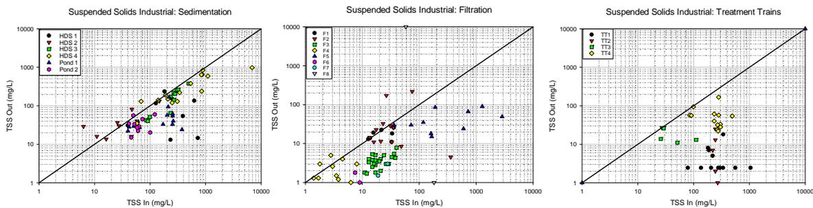
Figure 1. TSS removal in sedimentation (left), filtration (center), and treatment train (right) SCMs
