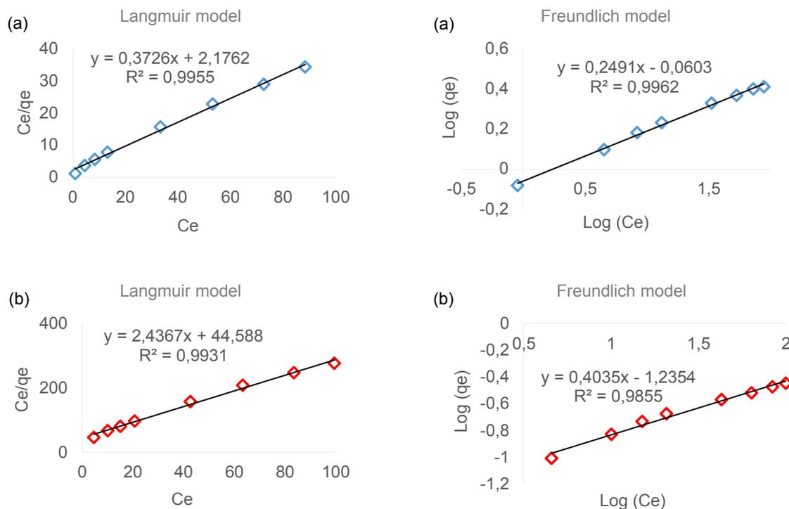
Fig.1. Langmuir and Freundlich models for sorption of Zn<sup>2+</sup> onto (a) the natural soil and (b) the synthetic soil.
