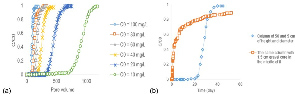
Fig. 2 (a) Zinc relative concentration versus pore volume for different influent concentrations for the natural soil (flow rate:  $50 \mu\text{L min}^{-1}$ ). (b) breakthrough curve for urban karst together with a simulation based on column experiments (influent Zn concentration:  $100 \text{ mg L}^{-1}$ , flow rate:  $1 \text{ mL min}^{-1}$ ).
