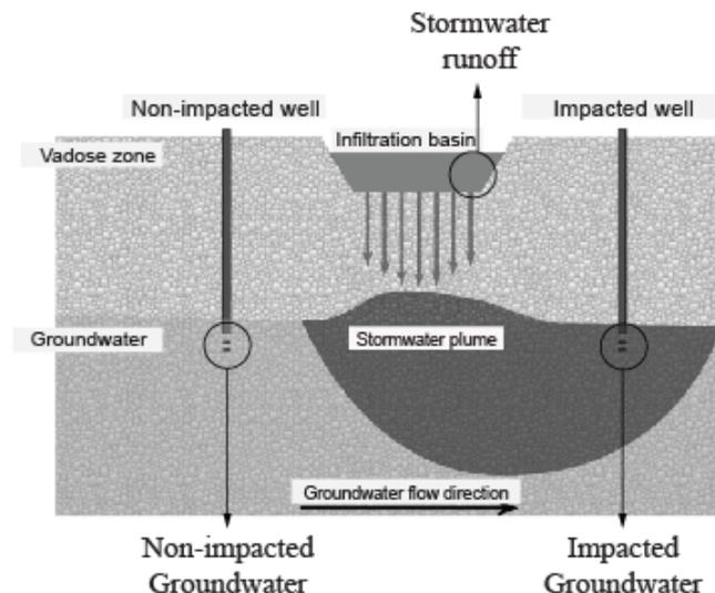
Figure 1: Positioning of sampling/incubation points in each stormwater infiltration system
