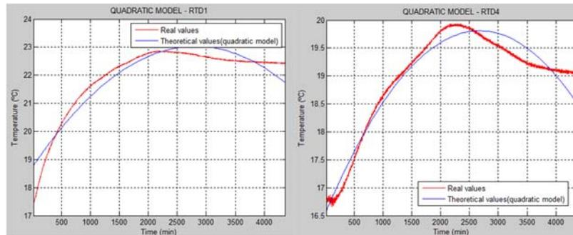
Figure 2. Quadratic models for the RTD1 and RTD4 for the pre-tests.
