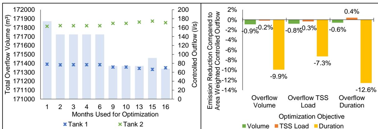
Figure 3 : Influence of length of measured input time series on optimized controlled outflow and total overflow volume (left) and influence of optimization objective on reduction of overflow volume, load and duration (right)
