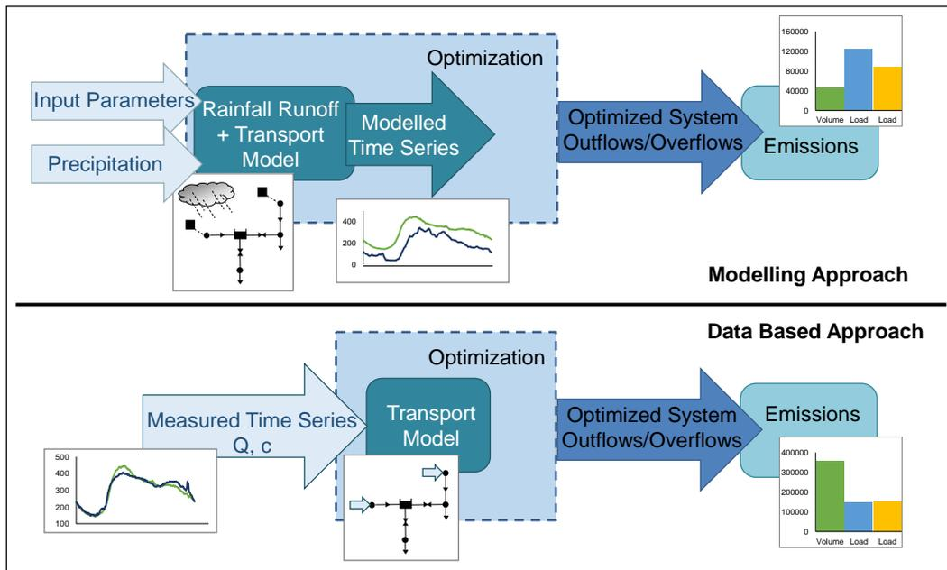
Figure 2: Conventional modelling approach for optimizing combined sewer systems and data based methodology in comparison; Q = flow time series; c = concentration time series
