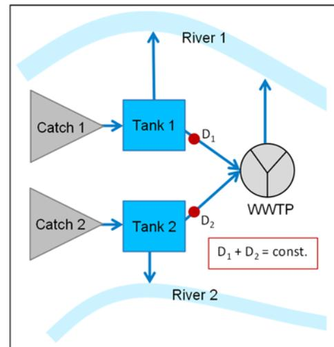
Figure 1 : Conceptual idealized catchment for data based system optimization; Catch = catchment, D = controlled outflow, WWTP = wastewater treatment plant
