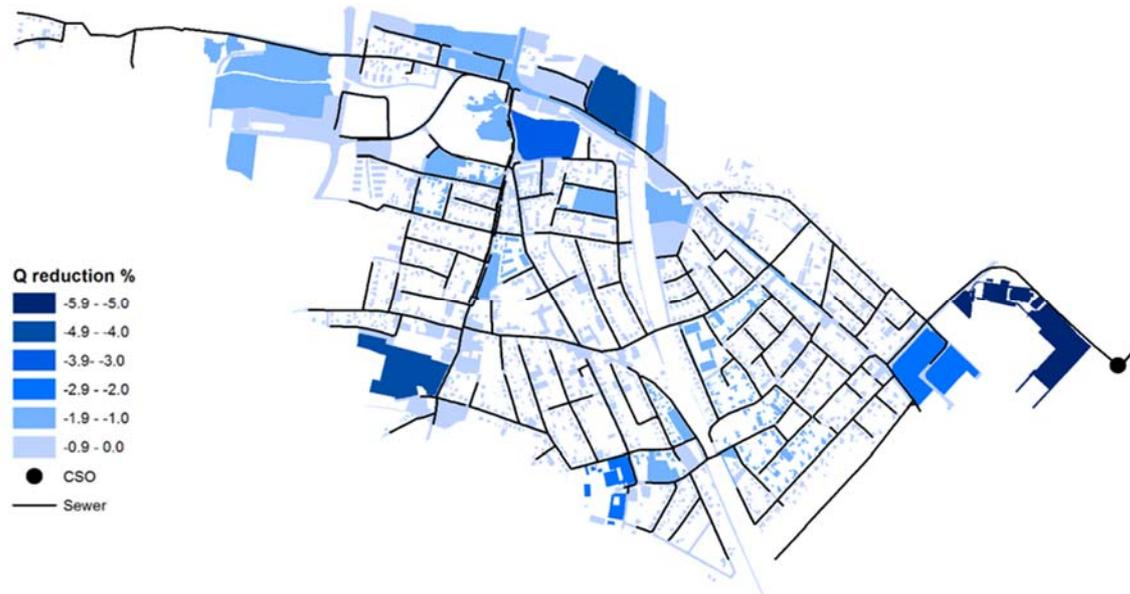
Figure 2 Reduction of CSO discharge volume in percentage
