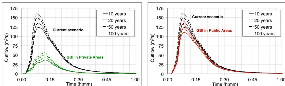
Figure 3: Outflow over time for precipitation events of 15 min and different recurrences at Flor d'Água catchment.
