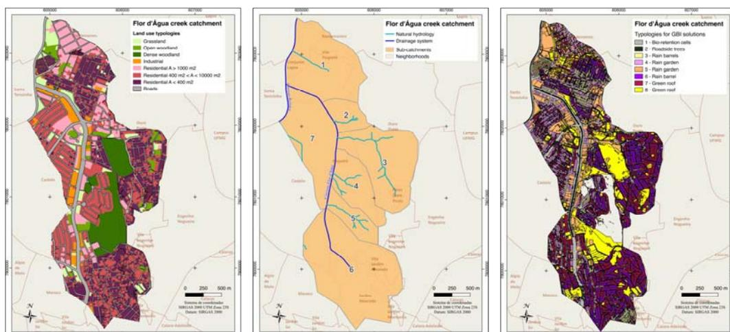
Figure 2 – Current land use and soil occupation of Flor d'Água catchment (left); sub-catchments used in the hydrological modeling (center); homogeneous typologies used to define GBI solutions (right).
